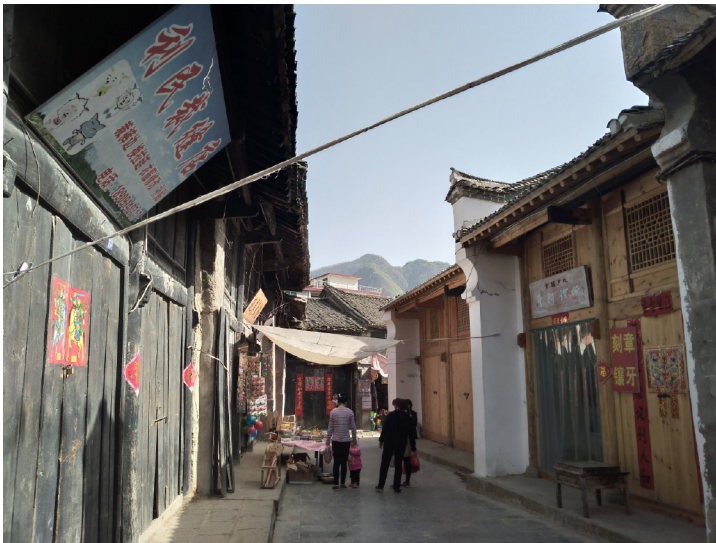
Fig. 5.10 A restored ancient building, the Matou Qiang has been covered with white plaster and the facades has been built with a natural finish wood.
