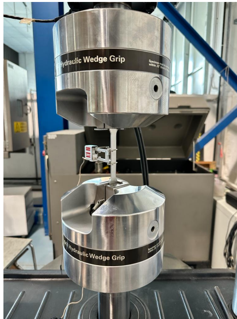
Figure B.1: Aluminum specimen mounted on machine
