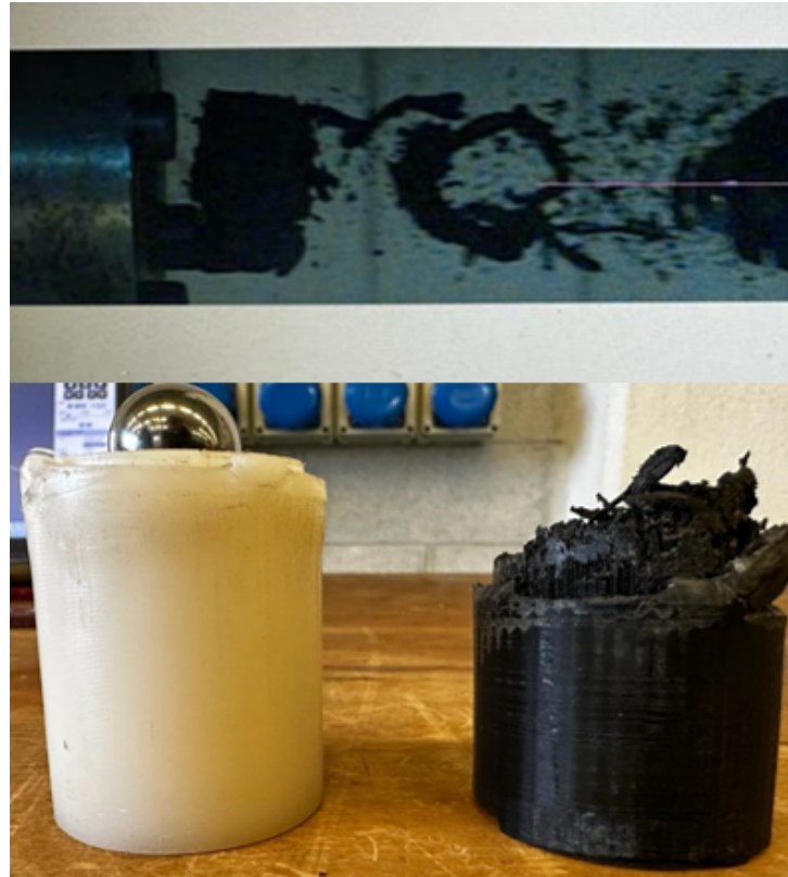
Figure 3.4: Top: Shot contaminated with destroyed PLA. Bottom: Comparison between two shot sabots, Nylon on the left and PLA on the right.
