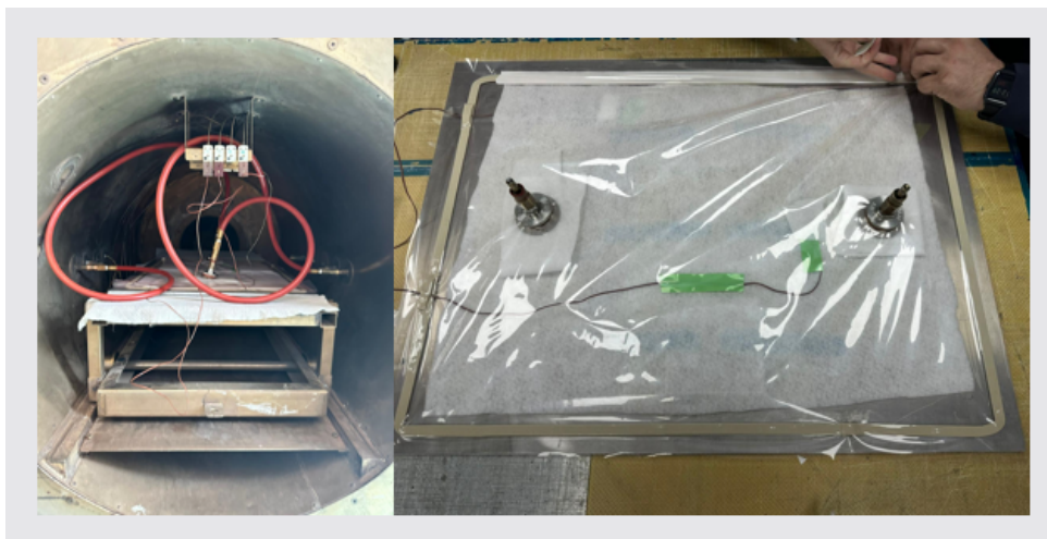
Figure 3.5: Vacuum Bag Manufacturing of Specimens
