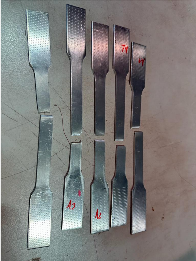
Figure B.3: Ductile failure of aluminum specimens
