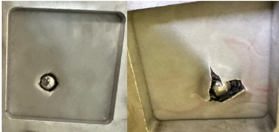
Figure 3.20: Impact test on specimen 3IFML
