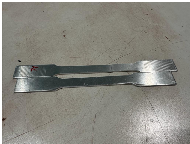
Figure B.2: Comparison failed specimen with undamaged specimen
