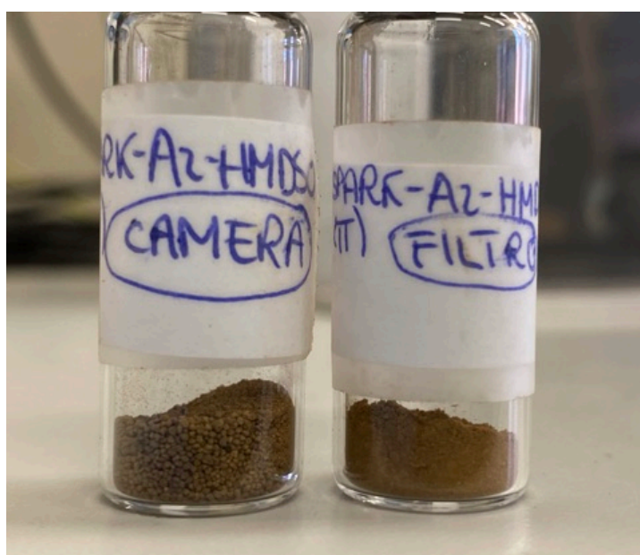
Figure 2.15 Plasma-treated lignin extracted from the chamber (left) and from the filter (right).
