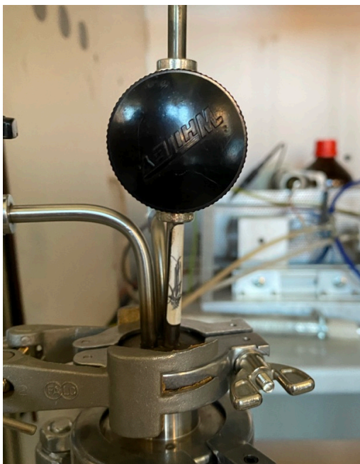
Figure 2.12 Rotating valve to open and regulate the gas flux of Argon or compressed air entering the liquid bubbler.
