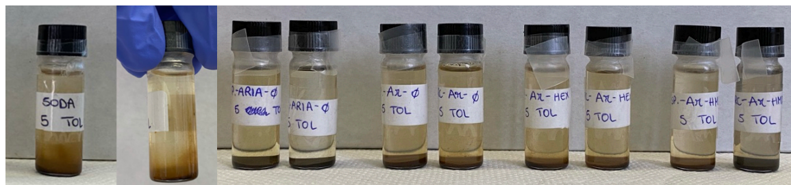
Figure 3.11 Solubility test of pristine lignin (two pictures on the left) and plasma treated lignin in toluene. In the picture on the right the plasma treated powders are divided in couples (spark on the left, arc on the right) and treatments are ordered as follows: air-0, Ar-0, Ar-HEX, Ar-HMDSO.
