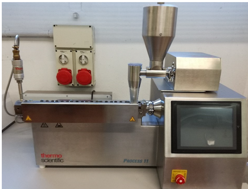
Figure 2.17 Process 11 parallel corotating twin-screw extruder by Thermo Fisher scientific
