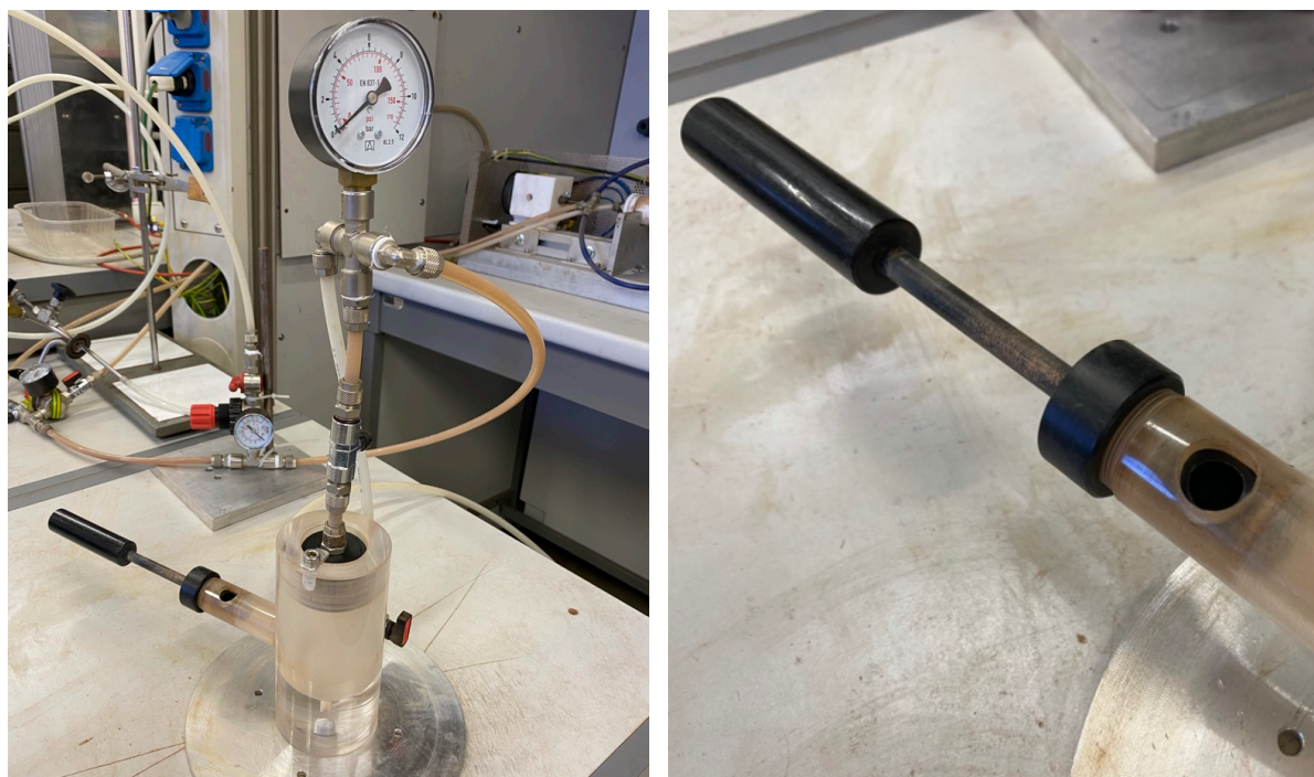
Figure 2.11 Powder injector (left) and zoom on the injection channel (right).
