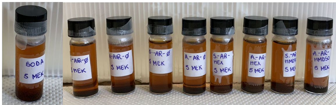
Figure 3.10 Solubility test of pristine lignin (left) and plasma treated lignin in methylethylketone. In the picture on the right the plasma treated powders are divided in couples (spark on the left, arc on the right) and treatments are ordered as follows: air-0, Ar-0, Ar-HEX, Ar-HMDSO.
