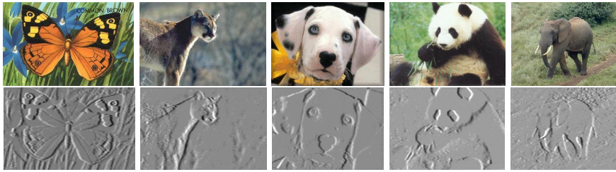
Figure 2.9: N-Caltech101 [116] samples. The first row shows RGB images from the original Caltech101 [142] dataset, while the second provides N-Caltech101 event conversions as voxel-grids.
