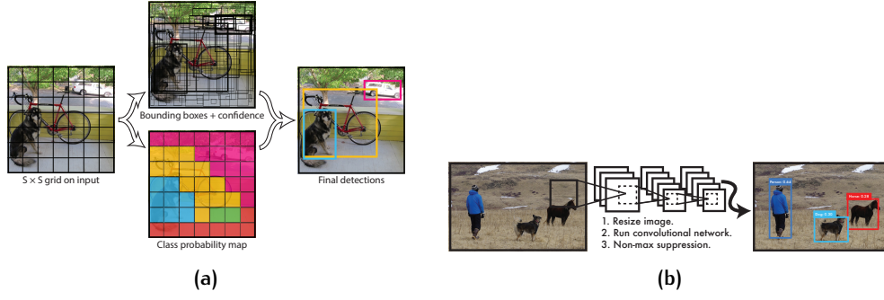
Figure 3.4: (a) The YOLO's bounding box prediction scheme. The image is first divided into a grid of S \times S cells, each predicting: a class probability (depicted on the bottom) and a set of boxes proposals, together with their confidence score (depicted on top with thickness proportional to the confidence). (b) The final set of predictions is obtained through non-maximum suppression and confidence thresholding. Figures taken from Redmon et al. [19]. Copyright ©2016 IEEE.
