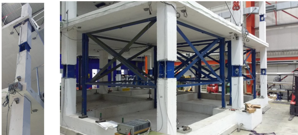
Figure 4.57 Safety measures, a) capitals at 1st floor and b) props on ground floor.
