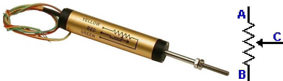
Figure 4.17 a) COD transducer b) Schematize of a potentiometer.
