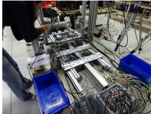
Figure 4.23 Sensors disposition for the calibration of box 1.
