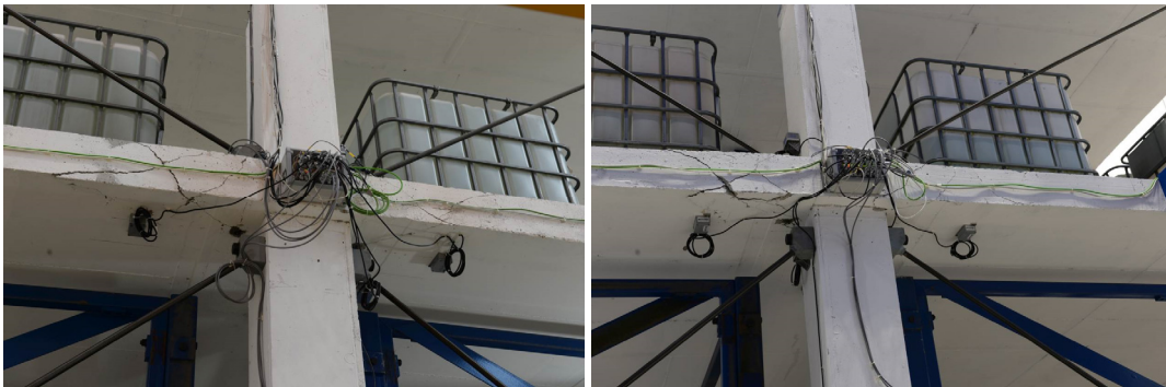
Figure 7.37 a) A2 and b) D2 connections after the 2% drift, tests Cyc-1 (f02).
