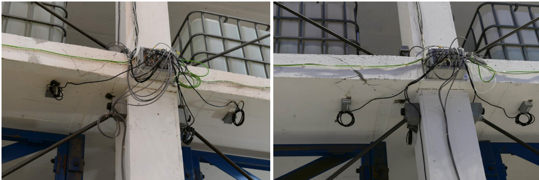
Figure 7.36 a) A2 and b) D2 connections after the 1.5% drift, tests Cyc-1 (f02).
