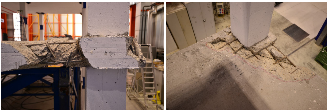
Figure 8.25 A2 connection after test Cyc-2 (g04), a) slab-column connection, b) slab west side.
