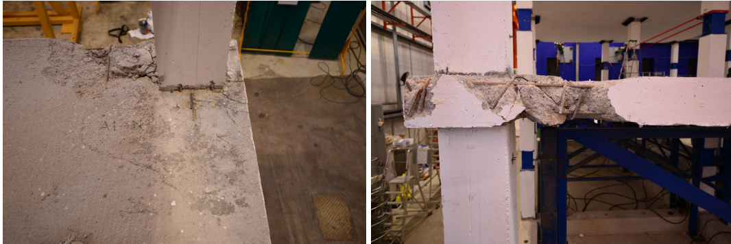
Figure 8.23 A1 connection after test Cyc-2 (g04), a) slab-column connection, b) slab east side.
