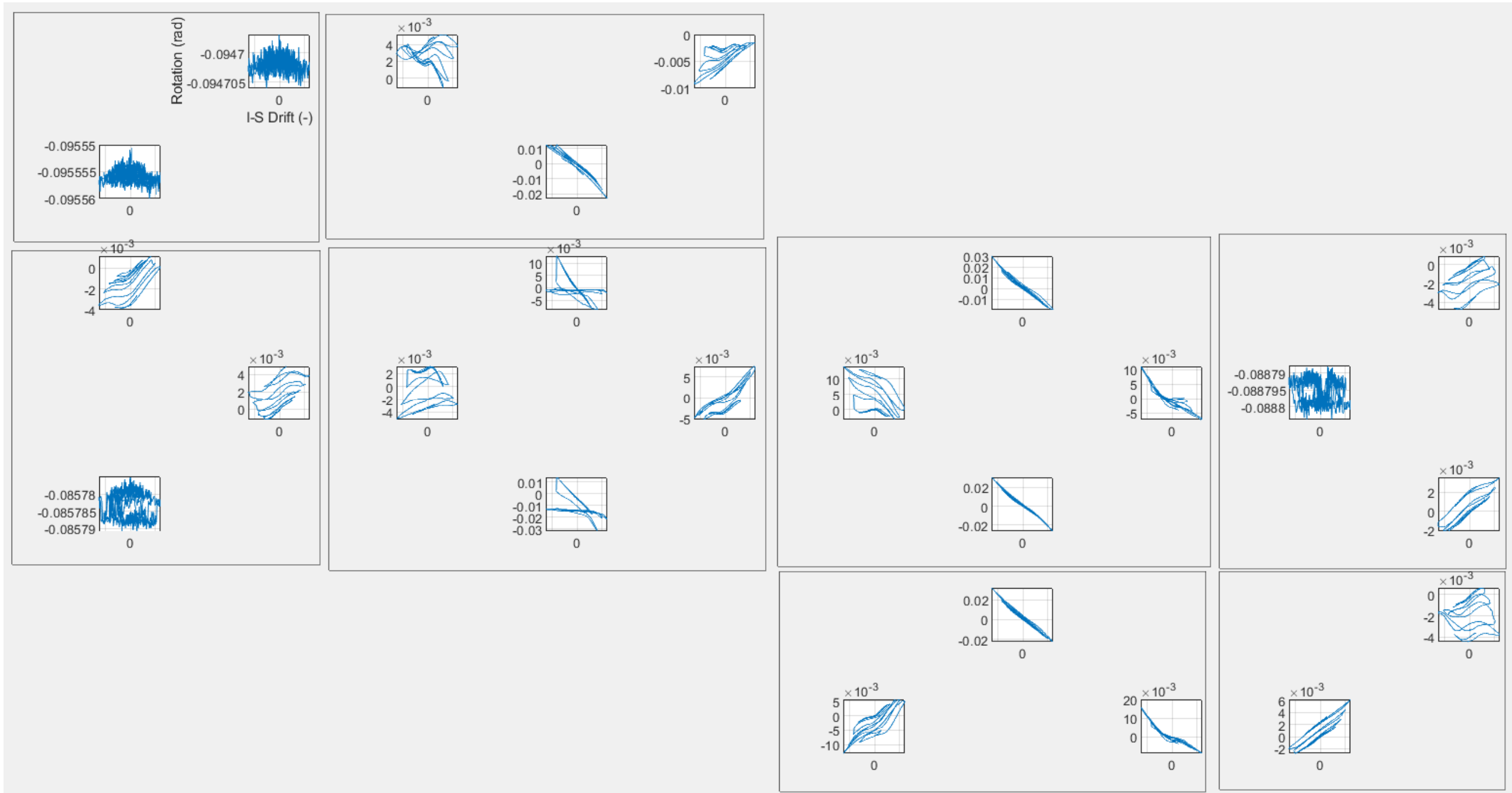
Figure 5.17 Slab rotation vs inter-storey drift ratio from each sensors in the 1 st floor, test Cyc-2.
